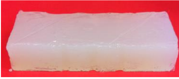
Fig. 2: A typical agar-based tissue-mimicking phantom.
