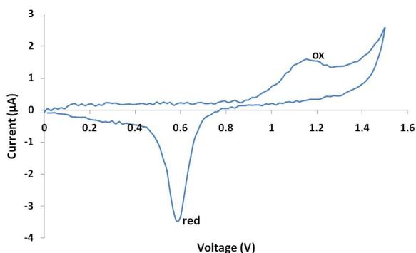
Fig. 4. Cyclic current-voltage curve of the Au W.E.
