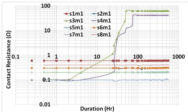
Fig. 8. Plot of ACA contact resistance vs. duration of humidity aging corresponding to the same electrode in all the 9 samples.
