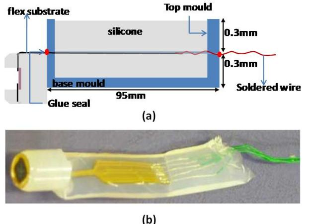
Fig. 5. (a) Cross-sectional schematic of the second encapsulation process and (b) picture of encapsulated sample for reliability testing.
