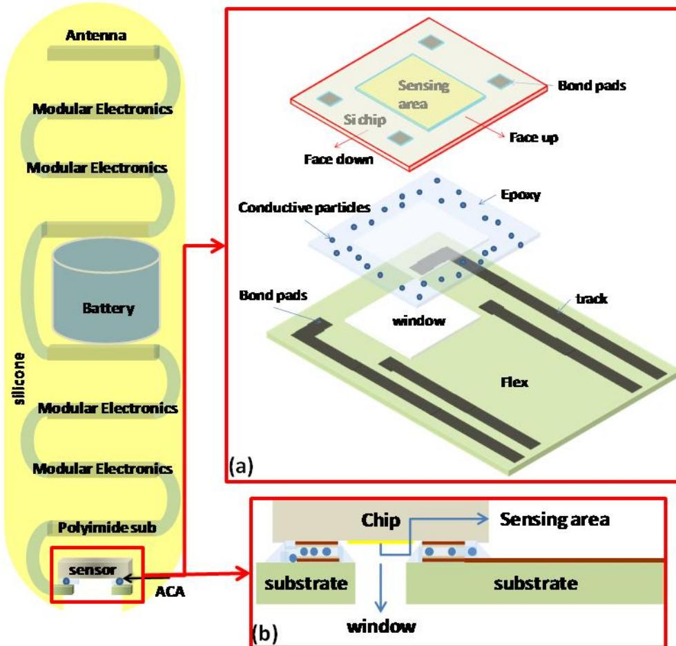
Fig. 1 Schematic of capsule with expanded image of FCOH (a) and (b) Cross sectional view of FCOC/DAS interconnections based on ACA
