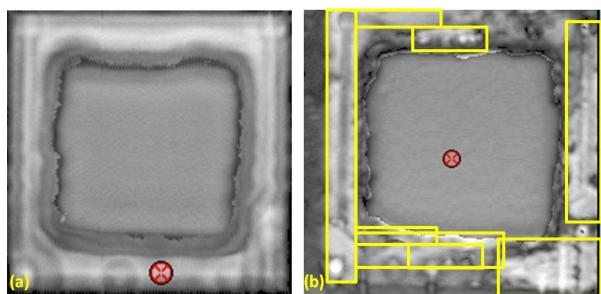
Fig. 11. SAM images (a) before and (b) after hygrothermal testing of one the samples that failed.
