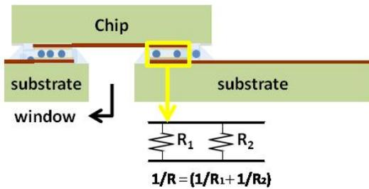
Fig. 7. Schematic of ACA interconnect showing the parallel configuration of the trapped conductive particles.
