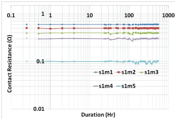
Fig. 6. Plot of ACA contact resistance vs. duration of humidity aging of all the electrodes in one sample.
