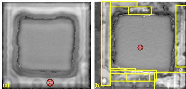
Fig. 11. SAM images (a) before and (b) after hygrothermal testing of one the samples that failed.
