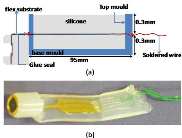
Fig. 5. (a) Cross-sectional schematic of the second encapsulation process and (b) picture of encapsulated sample for reliability testing.
