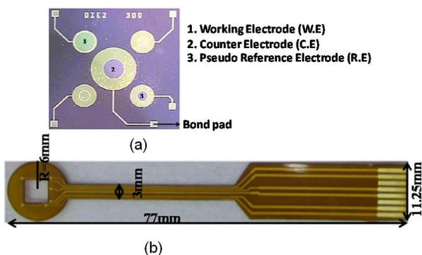
Fig. 2. (a) The direct access sensor chip and (b) Flexible substrate with window opening for sensor access.
