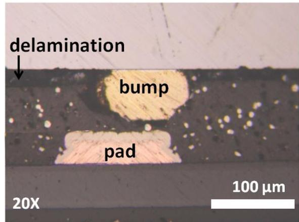
Fig. 12. Cross-section of samples after humidity testing - failure by crack propagation.
