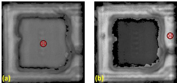
Fig. 10. SAM images (a) before and (b) after hygrothermal testing of one the samples that survived.
