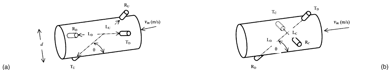
Fig. 2. (a) contra-propagation spool piece arrangement (transducers 90° out of plane) and (b) cross-flow spool piece arrangement (T: transmitter, R: receiver, L: ultrasonic path length, d : pipe diameter, v : fluid velocity; subscripts, C: crossflow, D: downstream, U: upstream).
